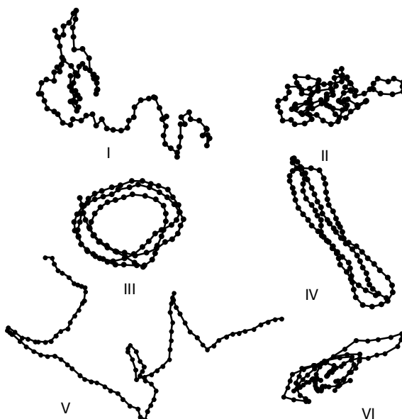
Figure 1 Typical conformations of a 100-segment homopolymer generated by Monte Carlo simulations. The simulation parameters are summarized in Table 1. They are
